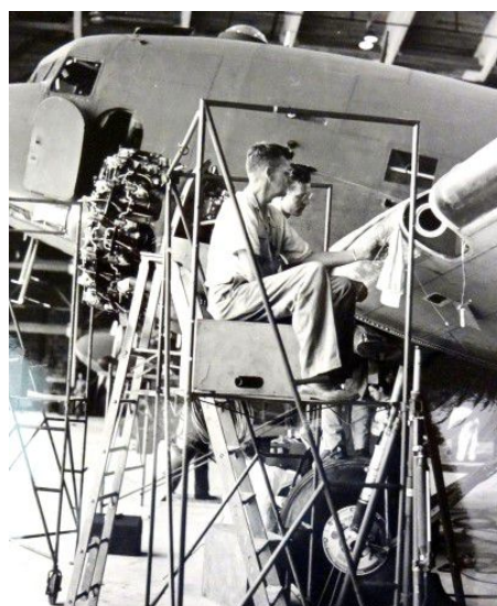
Northwest mechanics Alvin Smith and William Kuntz install de-icing equipment on a C-47 in Vandalia. Photo: Minnesota History Center Archives.
