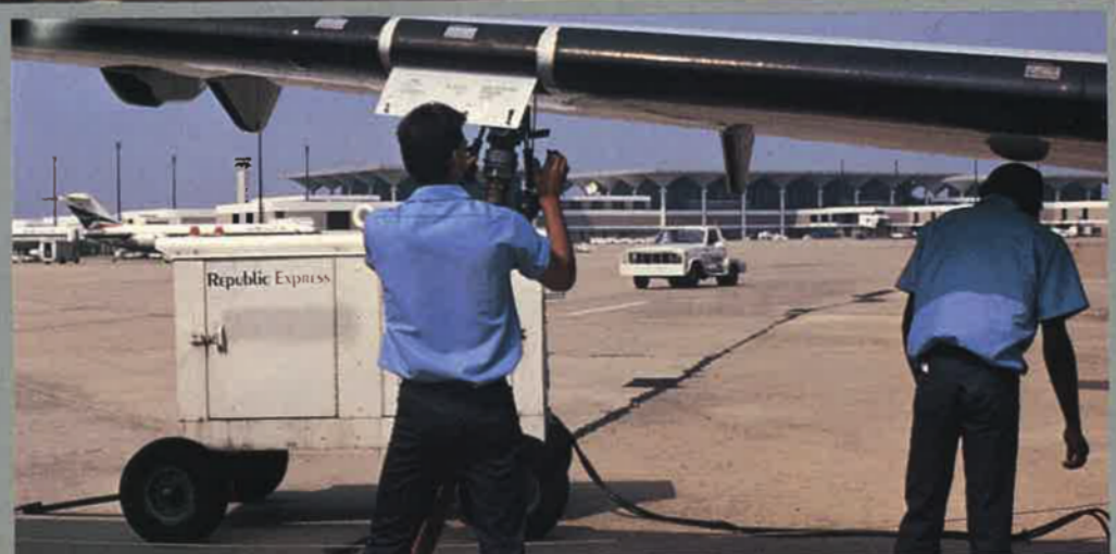
Underwing single-point pressure refuelling (overwing gravity refuelling is also provided) makes for quick turnarounds.
