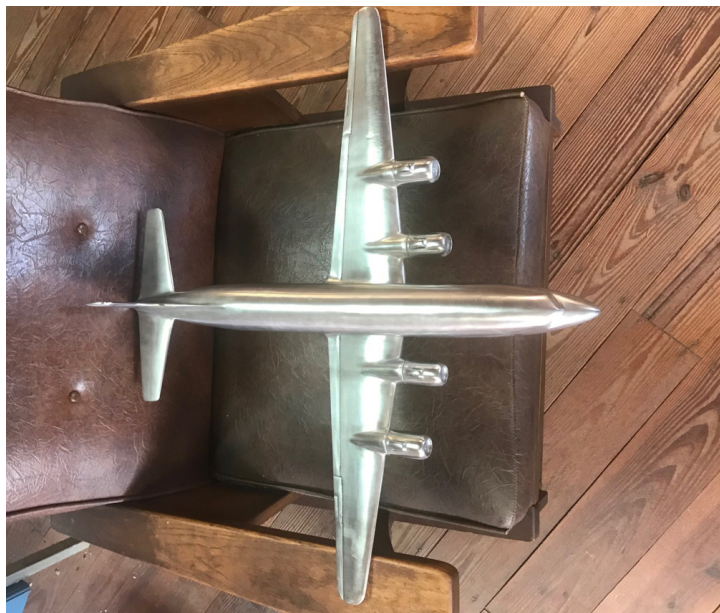
Striplin's photo from Sept. 27 shows the model stripped and wet-sanded, but not yet polished. New aluminum prop bushings had just been fabricated and installed in the engine nacelles.
