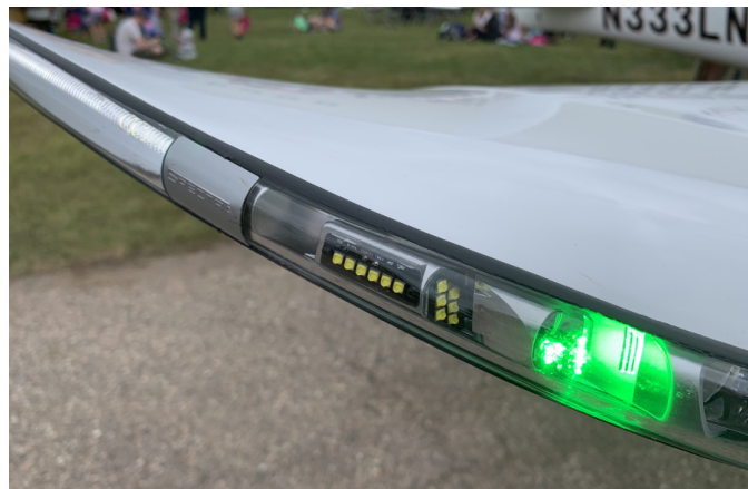
Wingtip strobe light installation on a modern Cirrus SR20, using LEDs. The entire assembly is only 1-1/2" top to bottom. Photo by author.
