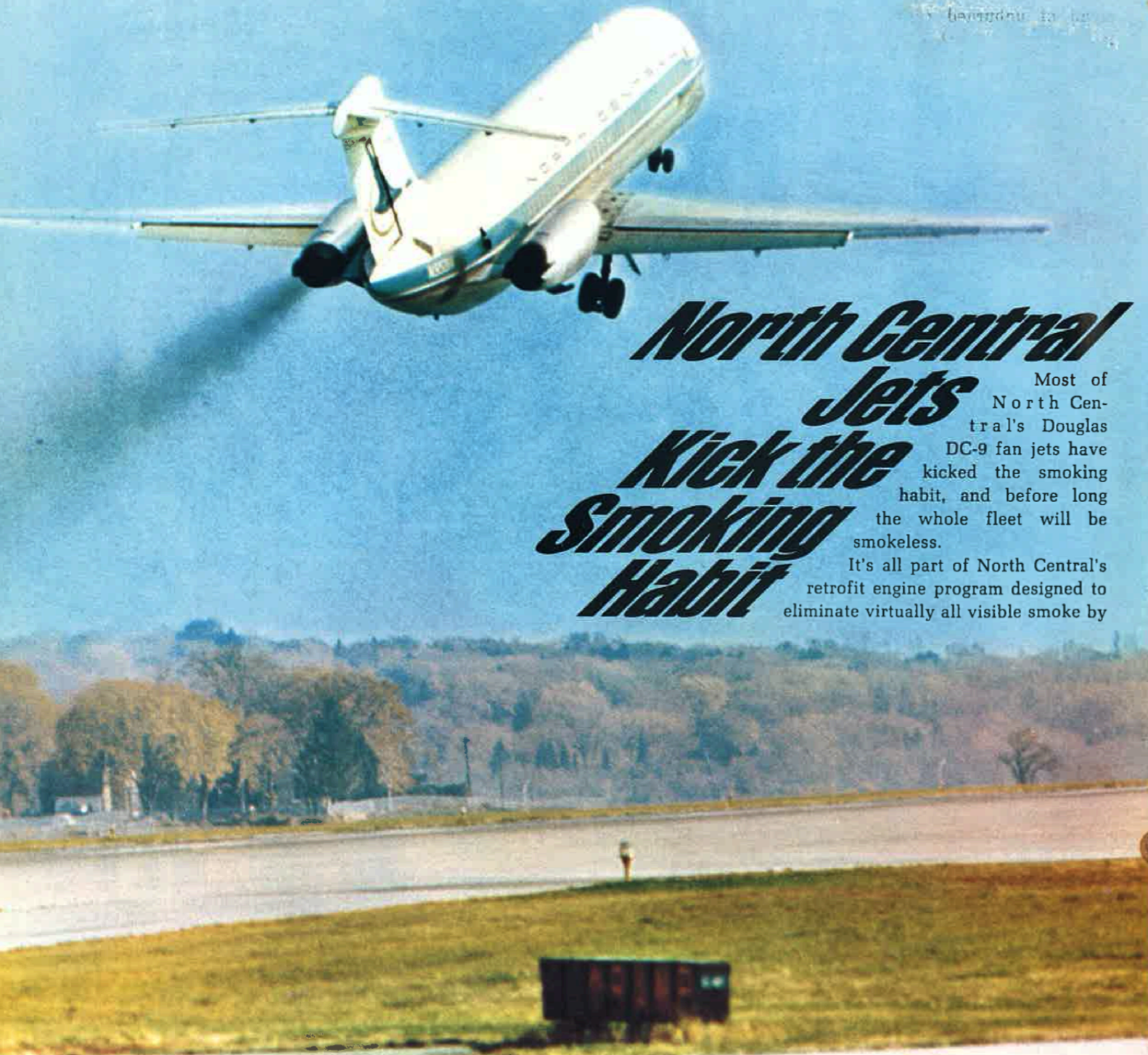
North Central DC-9 shows difference between engine with old burner can, left, and newly retrofitted engine on right.
