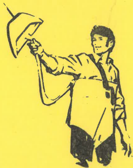
HOLD ONTO ESCAPE REEL. EVACUATE AIRPLANE THROUGH EXIT DESIGNATED BY CREW MEMBER. AVOID STRADDLING OTHER LINES.
