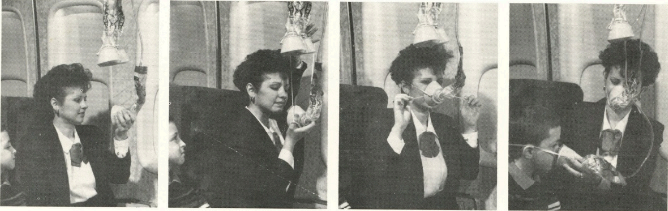
Quickly pull mask to activate oxygen flow. The bag will not fully inflate. Tighten mask for a secure fit.
