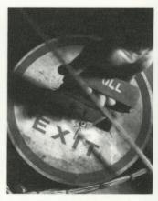
Located at the rear of the aircraft is either a plug hatch type or a pressure bulkhead door.
