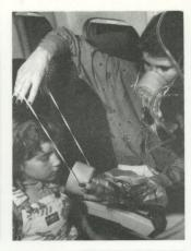
Quickly pull mask to activate oxygen flow. The bag will not fully inflate. Tighten mask for a secure fit.
