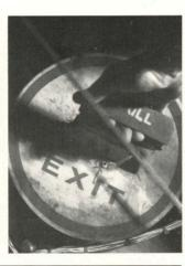
Located at the rear of the aircraft is either a plug hatch type or a pressure bulkhead door.
