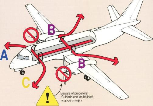
Assess outside conditions: If thick smoke, fire, metal debris or obstructions are visible, or if water level is above the sill of an exit, DO NOT OPEN. Redirect passengers to other usable exits.
