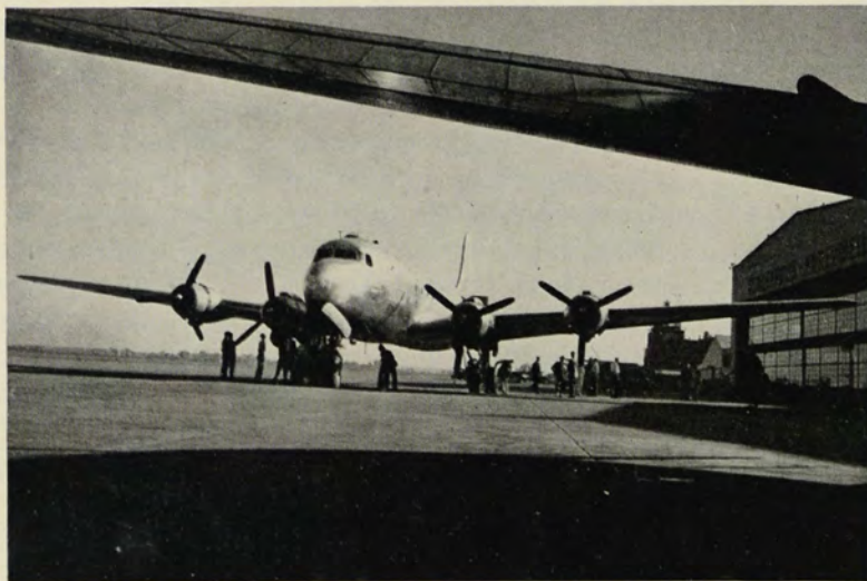
Forerunner of Northwest's fleet of four-engine transports is this C-54, leased from the Army for use in familiarizing pilots with the operation of these huge planes.
