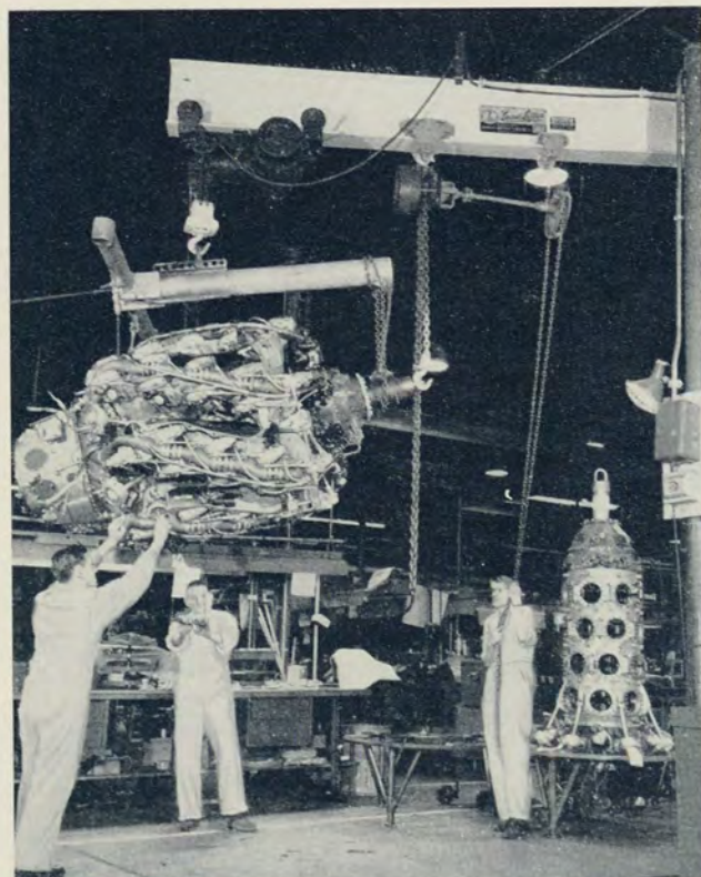
Overhauled Stratocruiser engine moves along. Crankcase (right) is ready for 28 new cylinders.
