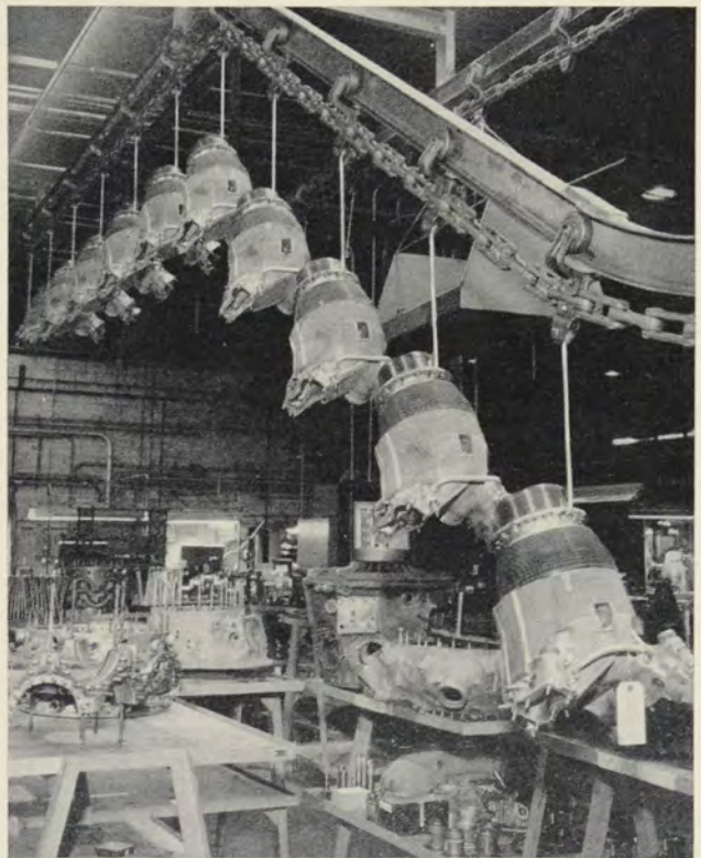
DC-7C engine cylinders move through overhaul base at St. Paul on new conveyor system.
