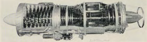
Northwest will be the first airline to operate DC-8C's equipped with the new, improved Pratt and Whitney JT4A-9 turbojet engine. The "A-9" develops 16,800 pounds of thrust, about 6 percent more than earlier JT4 models. Additional thrust provides improved take-off performance. Engine is more widely known by its military designation, J-75.
