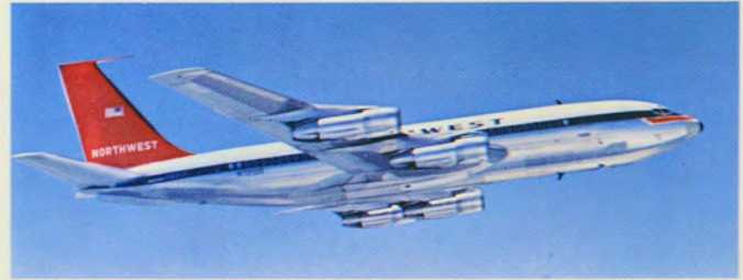
Boeing 720B Fan-Jets. Powerful. Versatile. Good for both long and short trips. Sixteen of these transcontinental Fan-Jets are flying Northwest passengers to major cities coast to coast. (Length: 130 feet, 6 inches—range: 4,430 miles—maximum speed: 606 mph.)
