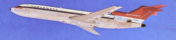
Your Company has ordered 16 Boeing 727-200 aircraft, with delivery of the first jet in November of 1968. The 727-200 retains all the proven features of the 727-100 and can be operated at a 20 percent lower seat-mile cost over routes of up to 1,500 miles. In addition, the 727-200 will carry 29 more passengers; has increased lower deck compartment space for additional luggage and mail, an improved braking system; and improved Pratt and Whitney power plants.
