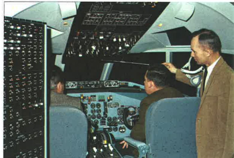
New DC-9 cockpit procedures trainer allows instructor to simulate aircraft conditions for flight crew's action.
