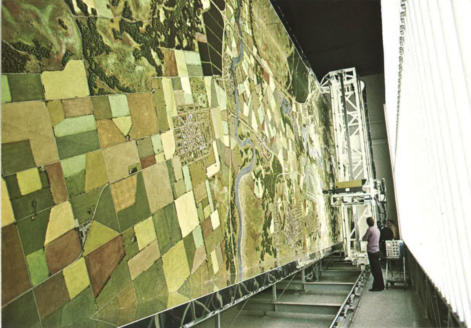
The most sophisticated flight simulator yet developed is the DC 10-40 simulator shown here, housed at Northwest Orient's flight services building in the Twin Cities. Heart of the closed circuit TV visual system is the terrain diorama, 60 feet long and 22 feet high.
