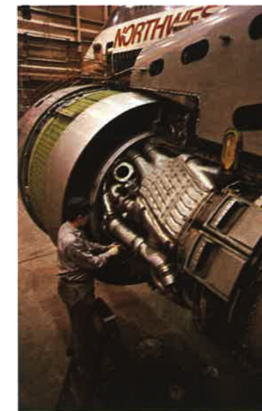
The same engine — the Pratt & Whitney JT9D — powers both NWA's 747's and DC 10's. This standardization gives the airline many savings in both time and expense. In these photos, two mechanics are completing overhaul of a JT9D engine while another performs a routine check on the engine on a 747.
