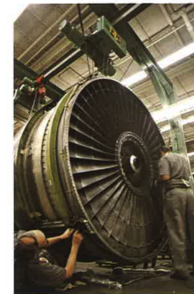
The same engine — the Pratt & Whitney JT9D — powers both NWA's 747's and DC 10's. This standardization gives the airline many savings in both time and expense. In these photos, two mechanics are completing overhaul of a JT9D engine while another performs a routine check on the engine on a 747.
