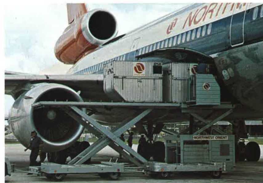
Automation is used increasingly in the airline industry. Here, LD-3 cargo containers are being loaded into the DC 10-40 by an NWA employee using a Clyde hydraulic loader. Use of sealed containers minimizes damage, provides greater security and increases ease of handling.
