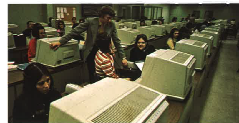
Northwest Orient's computerized passenger name record reservations system, called Insta-Res, is the most advanced in the industry today. Here, reservation sales agents at the Twin Cities general office are aided by miniature TV monitors which display complete information on the screen when called for by the operator.
