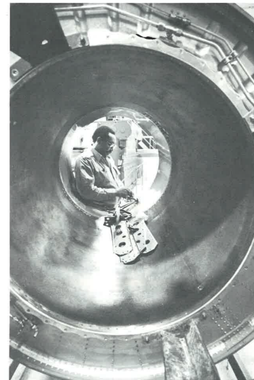
Skilled mechanics at Republic's Power Plant Facility perform all major maintenance on the company's JT8D jet engines.
