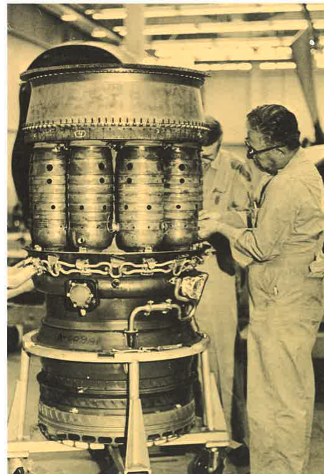
North Central mechanics are shown installing one of the nine new burner cans required to convert the JT8D fan jet engine to the low-smoke configuration.
