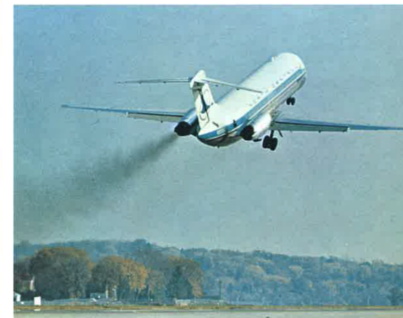
DC-9 Northliner demonstrates the substantial difference in smoke pollution between a conventional engine, left, and the engine on the right which has been modified with the air-cooled burner cans.
