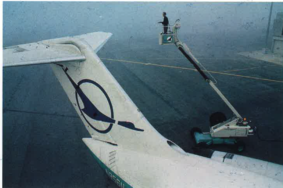
Vastly improved deicing systems are in service at the airline's major cold-weather stations. Snow and ice are quickly removed from aircraft, with minimum use of precious petroleum-based fluids.
