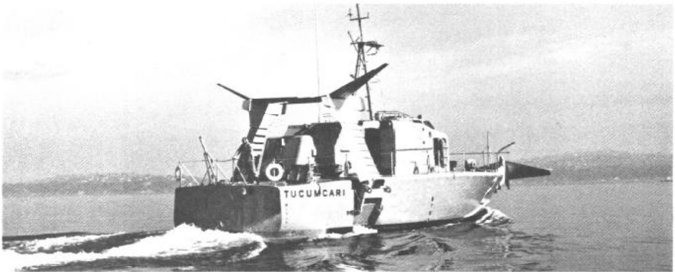
The 71-foot gunboat can attain speeds in excess of 40 knots. It is now undergoing Navy evaluation in the San Diego area
