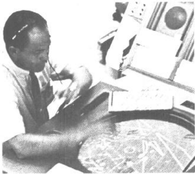
San Francisco tower controller follows inbound planes on final 15 miles of approach by means of televised radar screen.
