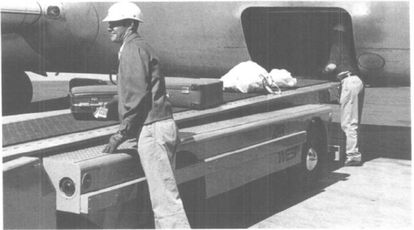
Phoenix agents Paul May and John R. Bennett find cargo handling almost a pleasure with new beltloader "Cargo King" conveyor is 22 feet long, 34 inches wide, with Ford 6-cylinder engine and transmission. It can handle up to 1,500 pounds
