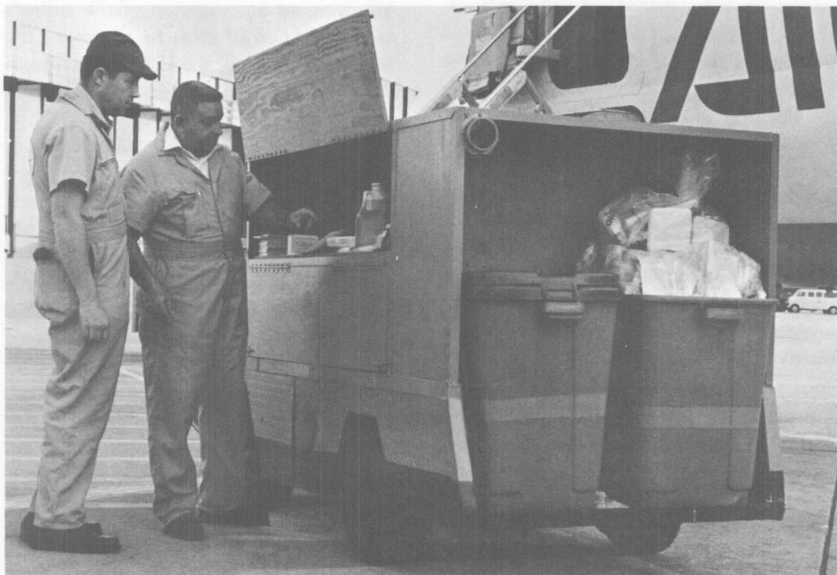
YANKEE INGENUITY — Los Angeles lead mechanic Harold Cumberlin, left, used slack maintenance periods to turn this scrapped electric ramp cart into a useful vehicle for aircraft cleaners. The cart, shown here with aircraft cleaner Ray Pedraza, was repaired and remodeled to be used by cleaners to haul their supplies and the trash taken from planes.
