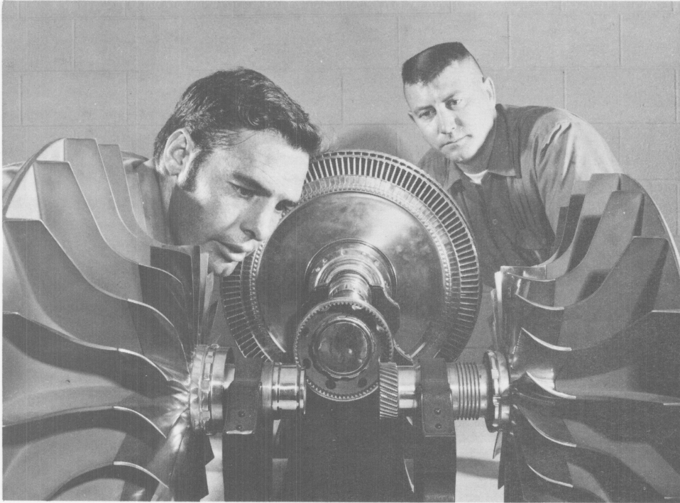
IT GOES VROOM! — Fan-like aircraft engine parts are examined by Phoenix mechanics Ray Files, left, and Neil Savage, who were undergoing recurrent training. The two centrifugal compressors flanking the engine turbine — resembling roulette wheels on edge — are vital components to the operation of the airline's F-27 aircraft.
