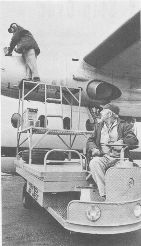
MECHANICS INVENTION — Mechanic Art Meyer, lower right, designed and built this maintenance service vehicle from a scrapped baggage cart. Mechanic Don Sailer, top left, uses the vehicle here to check the oil in a F-27 engine.
