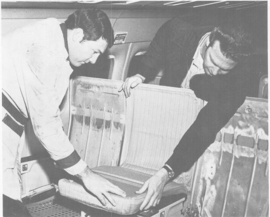
FOLD-DOWN SEATS — Fold-down seats are being installed in the company's DC-9 fleet. Two jets, N9330 and N9331, have been completed. The remaining aircraft will be converted by June 1. The conversion allows the back of the center seat in the three-seat row to be lowered and used as a tray for beverages, snacks or card playing. Ken Woodward (left), maintenance foreman, is checking the installation. Tom Arrowsmith, technician, is at the right. The missing seat cushions had been removed for cleaning.
