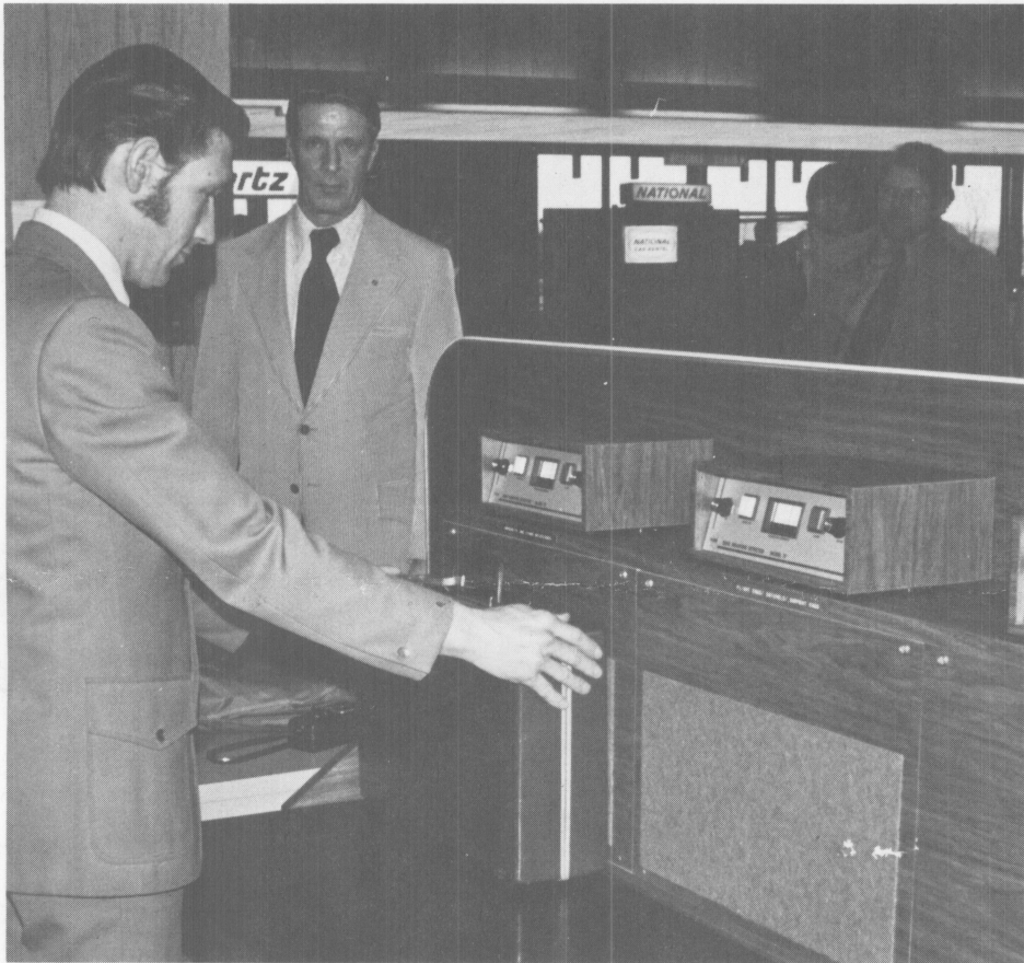
ELECTRONIC SEARCH — Hughes Airwest personnel in Eugene took part in a two-day test by the Federal Aviation Administration of the prototype of an electronic baggage search system. The new system, built by the Rens Corp. of Cottage Grove, Ore., would eliminate the necessity of opening baggage to search for weapons. Ron Spellmeyer (left), station agent, and Ed LeShane, station manager, were among those taking part in the test.
