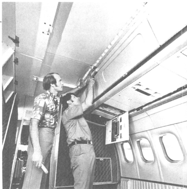
The first DC-9-30 with enclosed overhead storage modules entered scheduled service April 1. Checking finishing touches are John Walter (left), hangar maintenance manager, and Chuck Cumming, maintenance technician. All -30s are getting the compartments and new interior decor similar to our trijets. Renovation of each aircraft takes about seven days and is done in conjunction with C checks. Usable volume of each compartment is greater than those on many widebody aircraft. Loading capacity is 50 pounds.
