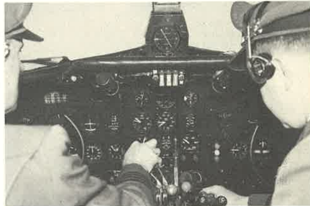
DC-3 pilot's cock-pit, showing dual instrument panels — planes are equipped for all weather night or day flying, including radar terrain warning indicator, static-free radio communication — cruise at three miles a minute. Twin quick-accelerating 1200 h.p. engines — maintain flight on either engine alone.
