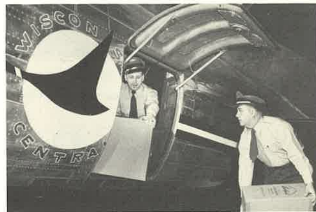
Specially built cargo hatch and compartment speeds handling of baggage and cargo. Hatch opening 2 ft. 7 inches x 3 ft. 10 inches to accommodate bulky packages.
