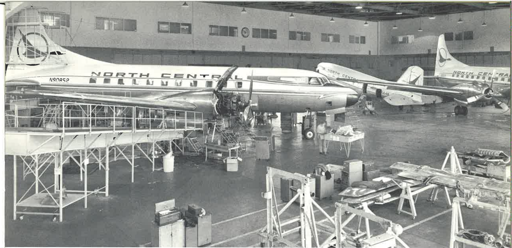
A newly-acquired hangar at the Minneapolis/St. Paul main operations base now provides over 30,000 square feet of floor space for line maintenance and 8,000 square feet of office space. A work dock, shown at left, greatly facilitates Convair maintenance.
