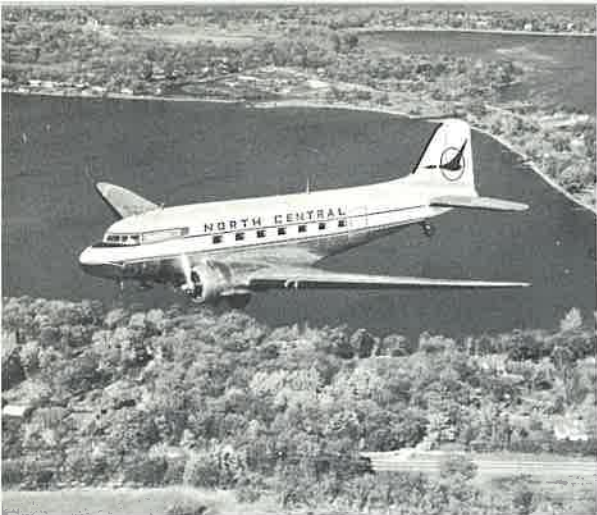
The venerable, reliable Douglas DC-3 made scheduled airline service possible. North Central operates 29 of these aircraft over its 7,000-mile system in 10 states and Canada. The DC-3 Northliner carries 26 passengers and a crew of three, and cruises at 180 miles an hour at 10,000 feet.
