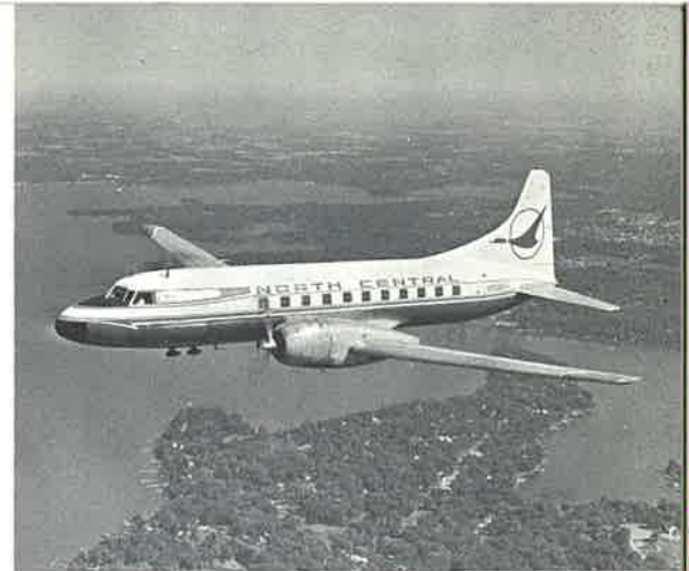
The Convair 440 Super Northliner, luxury aircraft of the North Central fleet, provides air conditioned, pressurized cabin comfort for its 44 passengers. Cruising at 289 miles an hour at 20,000 feet, the Convair is equipped with weather radar and high-intensity Honeywell-Atkins Maximum Safety wingtip lights. The company operates 18 Super Northliners.
