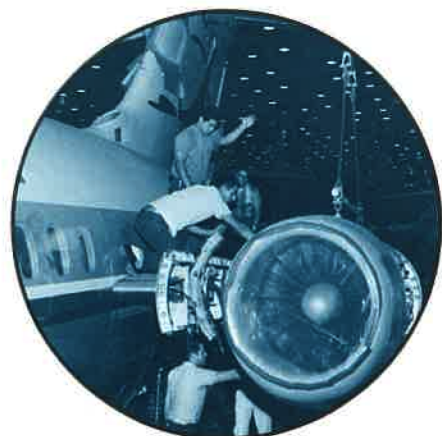
DELICATE PROCESS — A Pratt & Whitney fan jet engine is slowly and carefully moved into position on the rear fuselage of the DC-9. Powered by two JT8D-7 engines, the aircraft cruises at 560 miles an hour.
