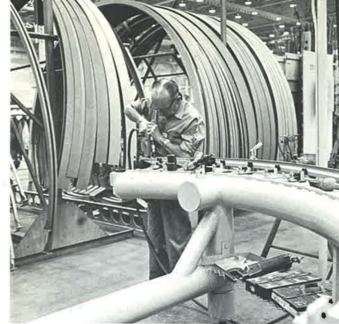
THE BEGINNING — A workman starts the assembly of a fuselage section for North Central's first DC-9 jetliner with a curving frame installed on a carefully aligned jig.
