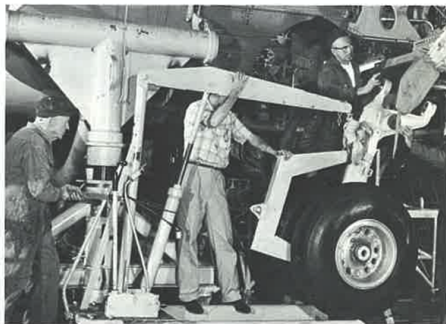
LANDING GEAR —One of two main landing gear for the DC-9 is installed on the final assembly line. Prior to getting its own wheels, the DC-9 is supported by mobile hydraulic devices.
