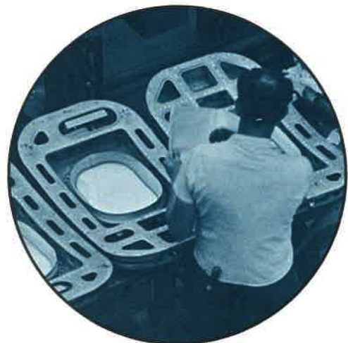
FINAL CHECK — Before installation, the DC-9 emergency exit doors are given a final examination. Each DC-9 Series 30 has four such doors, two on each side, located amidship over the wings.
