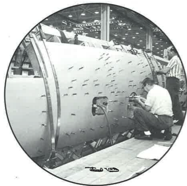
PRECISE WORK — Douglas workmen are shown riveting a portion of the DC-9 fan jet fuselage.
